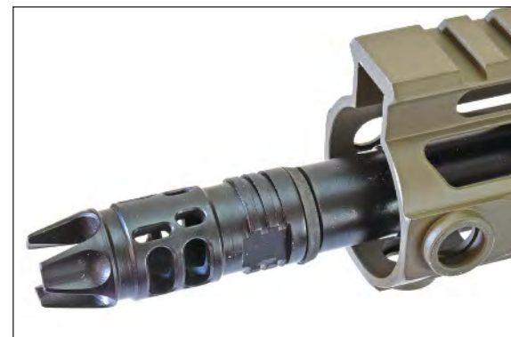
The EvoIV muzzle device from MFT is meant to be a combination muzzle brake and flash hider. Tarr found it was a very effective muzzle brake, but didn't do much to kill flash.
