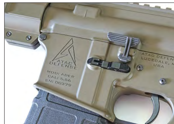
The bolt catch is a unique design that works either for releasing the bolt or helping to lock it back. Below it you can see the left-side magazine release.
