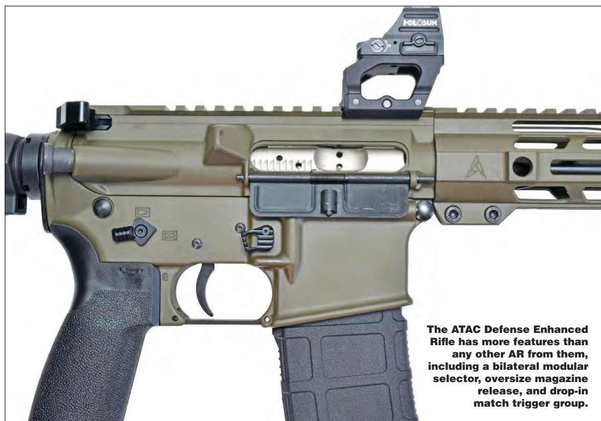
The bolt catch is a unique design that works either for releasing the bolt or helping to lock it back. Below it you can see the left-side magazine release.
